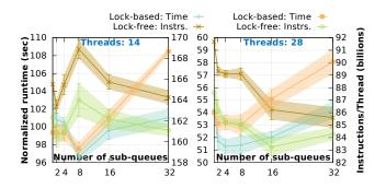
Figure 7: Comparison of lock-based vs. lock-free Interthread Event Queues (ITEQs)
