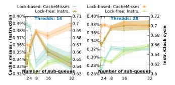
Figure 8: Lock-based vs. lock-free ITEQs: Instrctions/CPUcycle & cache misses
