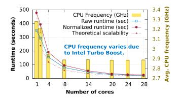
Figure 2: CPU frequency changes due to Intel<sup>®</sup> Turbo Boost & runtime normalization
