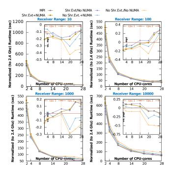
Figure 10: Config #1: Comparison of normalized runtimes. Inset charts show percentage difference versus MPI, with positive values indicating speed-up
